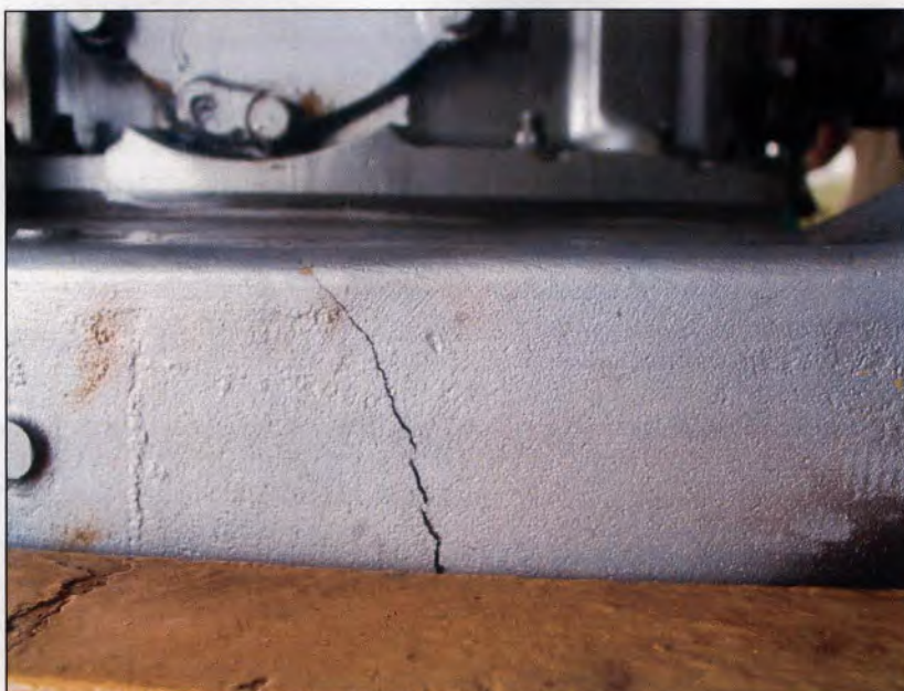
Figure 35 – Foreign military support case crack (2006). (Picture Source: Bell)
