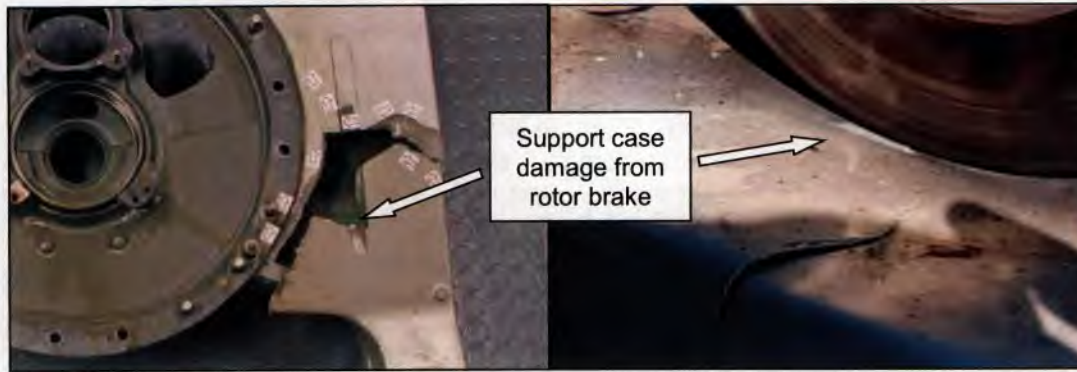
Figure 45 - Two examples of rotor brake contact with main gearbox support cases during an accident.
