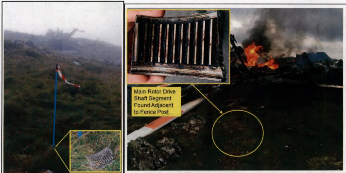
Figure 8 - Forward outer coupling fragments found in relation to the aircraft wreckage. (Picture Source: DAIB report)
