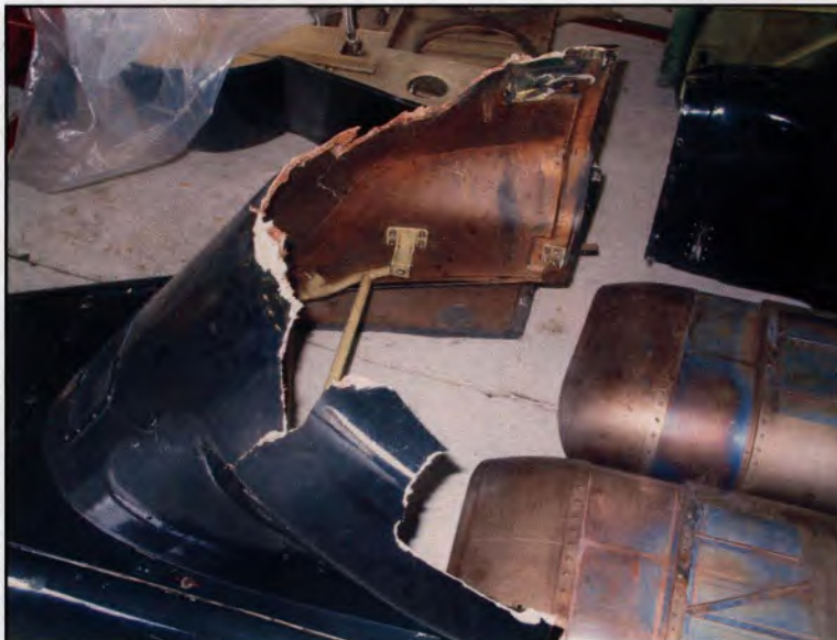
Figure 25 - Forward upper cowling debris from similar Bell 412 accident, showing damage as a result of pitch change links impacting the cowling. (Picture Source: Bell)
