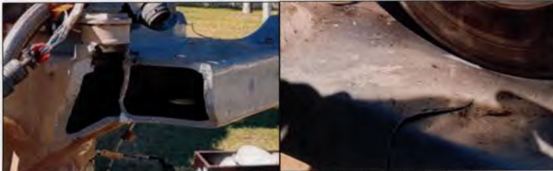
Figure 37 – Damage to the support case in the Australian accident (2017).
