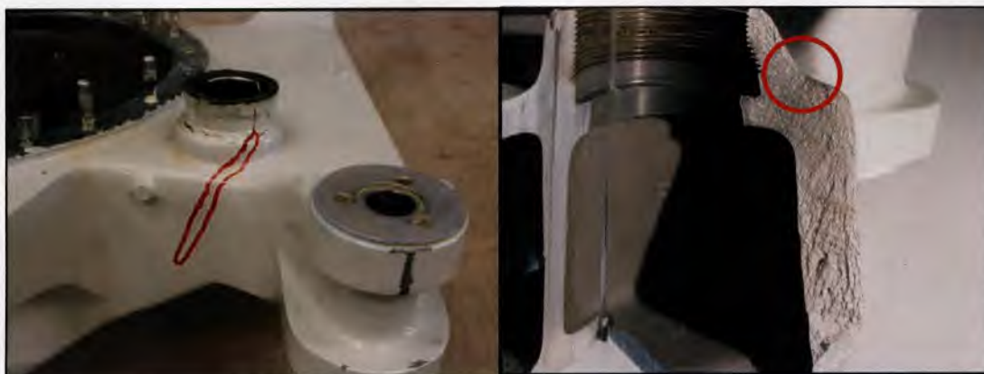
Figure 32 – Images from the Bell engineering laboratory report on the fatigue crack found within the support case of ZJ241 in 2006. [Left] Location of the fatigue crack on the support case. [Right] Fatigue crack surface showing the initiation site in the circle. (Picture Source: Bell)
