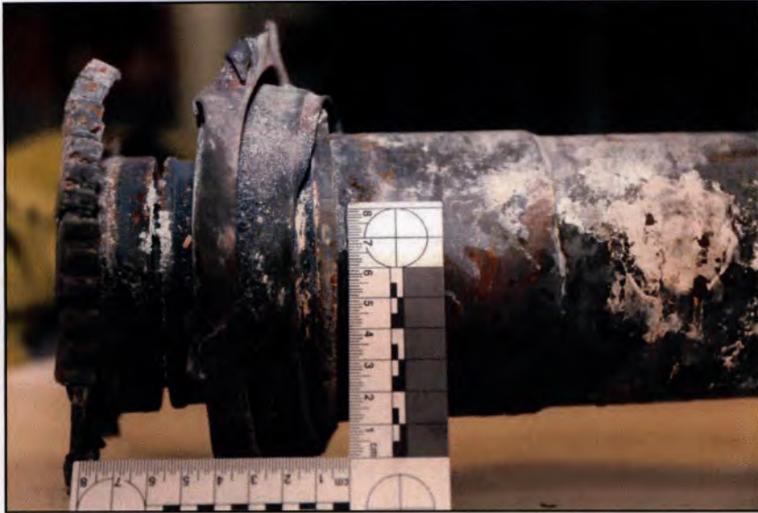
Figure 21 - Forward inner coupling including oil boot. (Picture Source: 1710 NAS)
