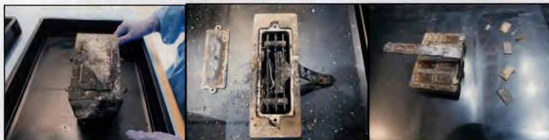
Figure 12 – [Left] CVR condition on recovery. [Centre] Memory module assembly. [Right] Three layer integrated circuit board and loose components.
