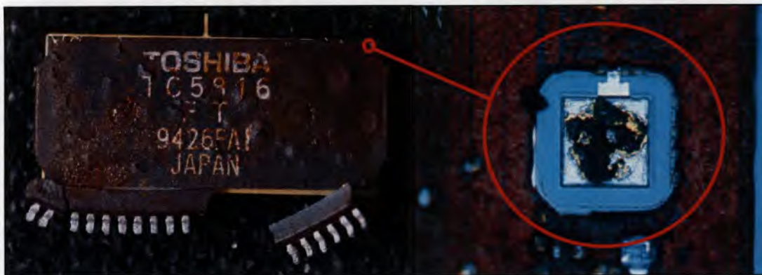
Figure 13 – [Left] Showing one of the damaged chips with partially de-packaged casing after recovery action and [Right] Showing a high magnification image of a damaged bond pad. (Picture Source: DSTL Chip Damage Analysis Report.)
