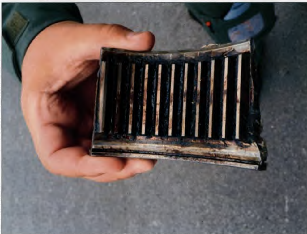
Figure 4 - Fragment of driveshaft coupling found by the awaiting Passenger. (Picture Source: Passenger)
