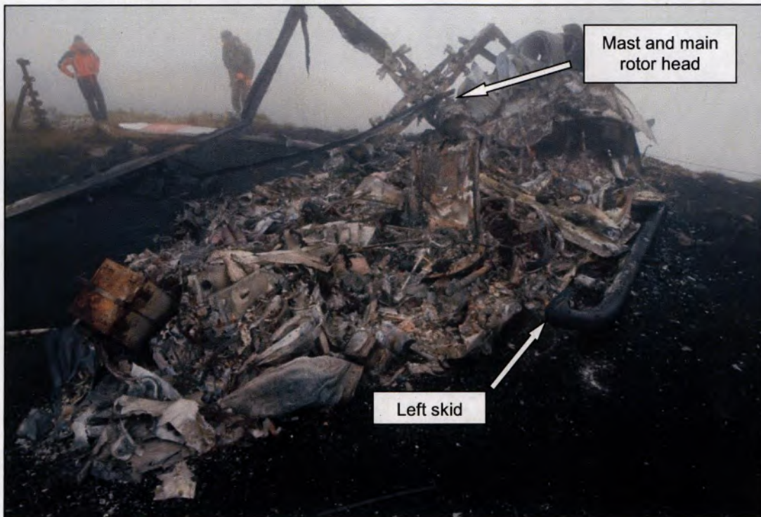
Figure 7 - Aircraft wreckage and immediate surrounding area. (Picture Source: DAIB Engineering)
