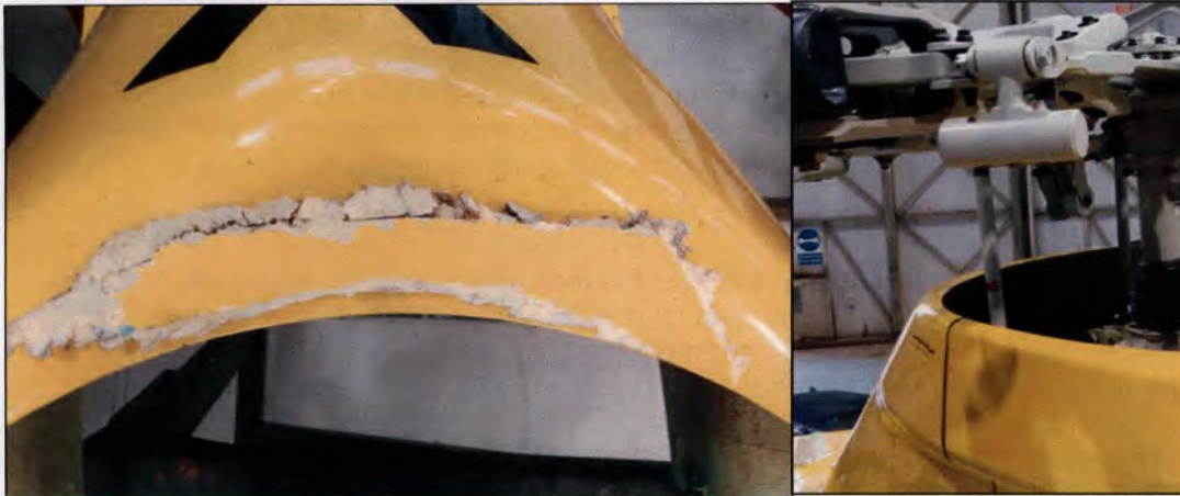
Figure 24 – [Left] Cowling debris shown from above, overlaid on a serviceable component. [Right] Showing the relative position of the pitch change links to the cowling. (Picture Source: DAIB Engineering)
